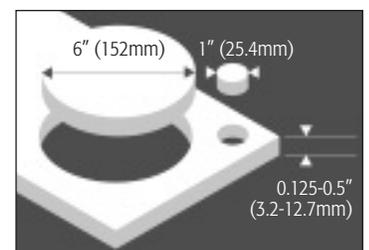
Cuts foamboard or cellfoam circles from 1" to 6" diameters (25.44 to 152mm), and depths from 1/8" to 1/2" (3.2 to 12.7mm).
