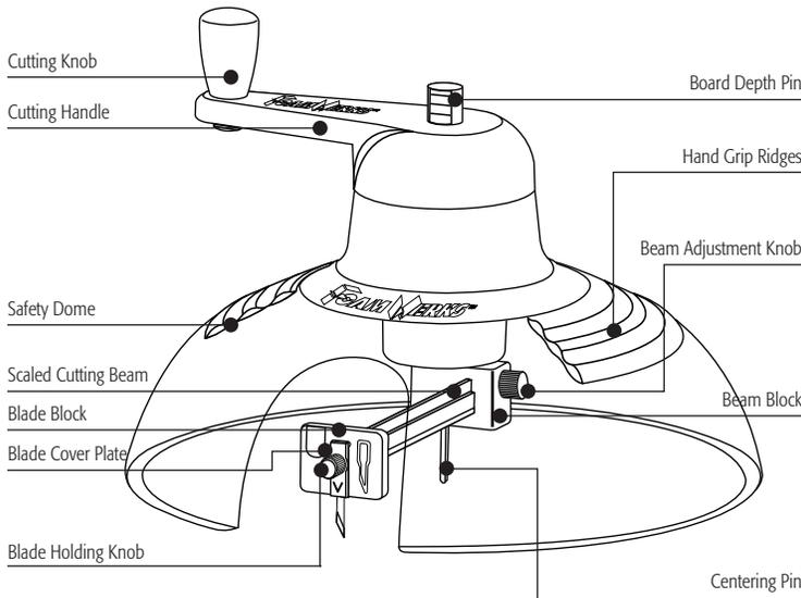
**Cutting Knob** - Knob attached to the Cutting Handle, used to turn the Scaled Cutting Beam and Blade
